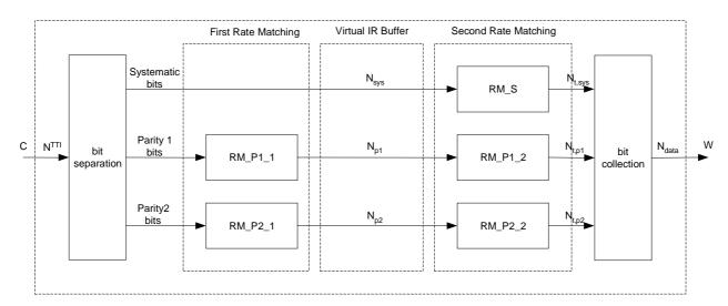
Figure 17: HS-DSCH hybrid ARQ functionality
